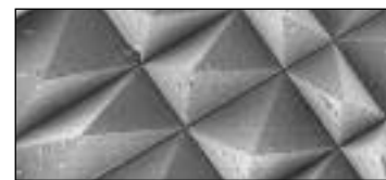
The precisely structured surface of Trizact™ film is clearly visible under 50X magnification
